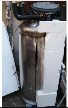
DHW tank rupture and water leak
