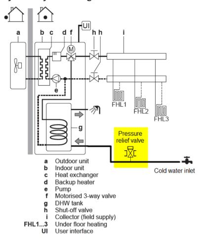
Note: the above layout is a modified and simplified diagram for the Daikin Altherma LT floor-standing (integrated) unit, however, the requirement of the pressure relief valve is applicable for all DHW circuits connected to any Daikin product.
